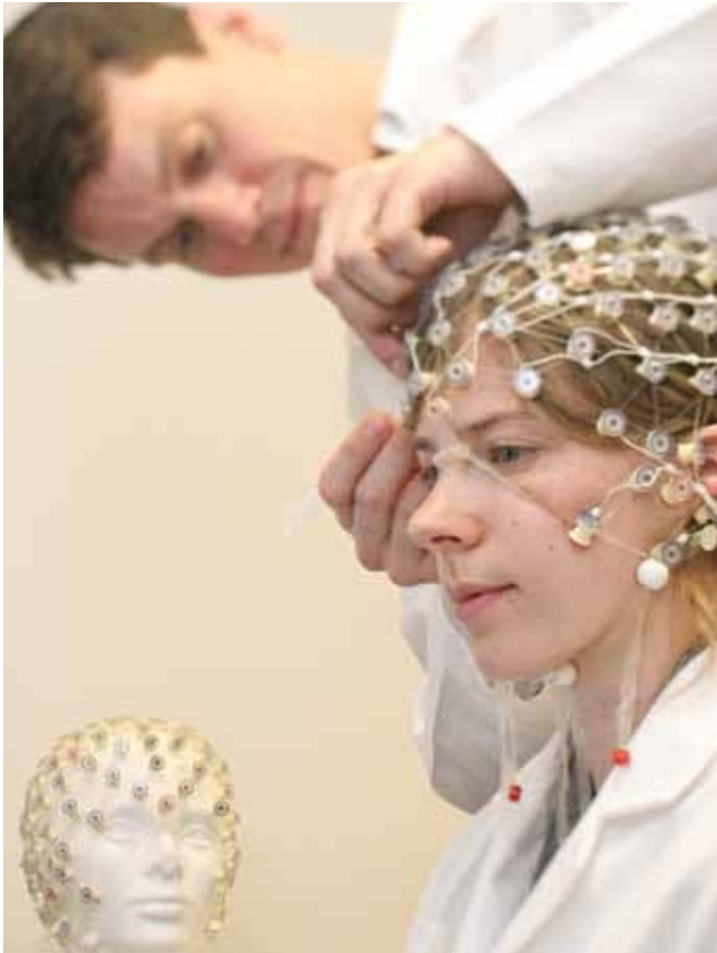
In EEG, electrodes placed around the head record electrical activity of the human brain in response to a variety of stimuli and activities — even sleep.
